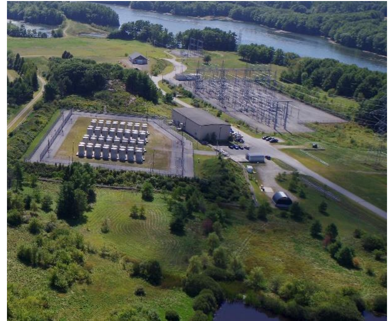
Dry-cask storage facility at now-decommissioned Maine Yankee nuclear power plant in Wiscasset, Maine.
